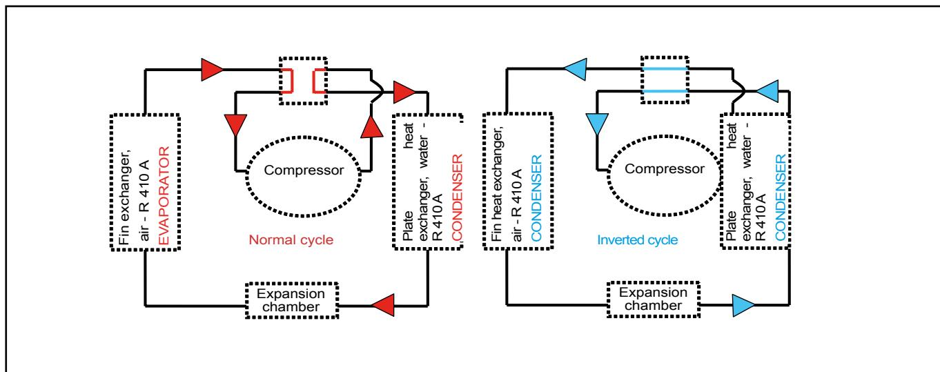
The roles of the evaporator and condenser are reversed: The fluid brings calories to the fin heat exchanger to melt the ice. The fan remains stopped while the system is defrosting. When the temperature detected by the sensor increases, defrosting is finished and the 4-way valve switches back to the normal cycle.
