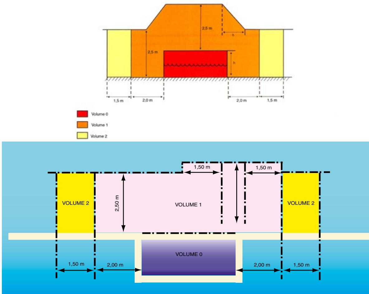
**Volume 0:** Safety extra-low voltage\* (SELV) < 12 V alternating or 30 V direct + the equipment must be IPX8 rated (dust-free, waterproof).
