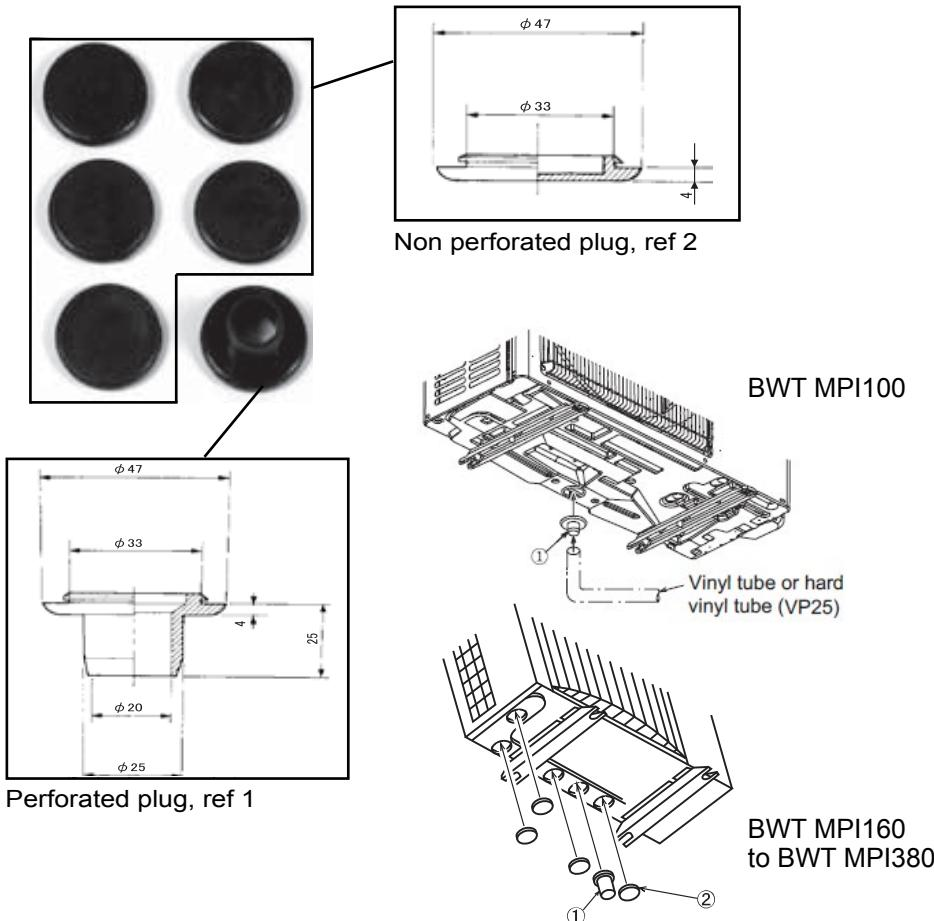
The plugs should be inserted in the holes in the base of the machine, see the figure opposite. Note that the perforated plug (ref 1) should be located at the lowest point to allow the condensates to drain properly.
