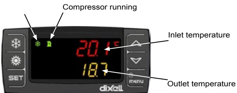
The following information is displayed when the machine detects an anomaly.
