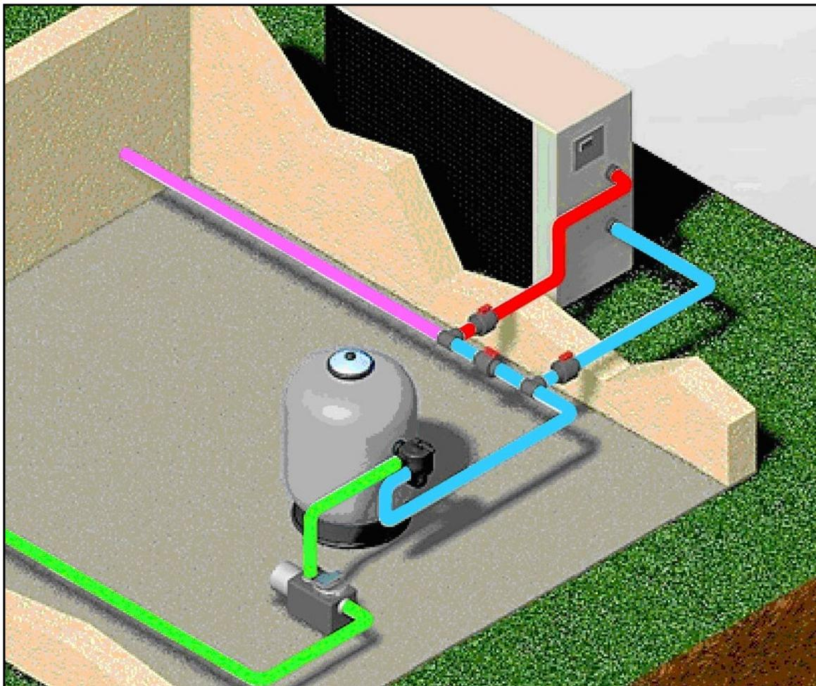
The pipes, valves and unions constituting the by-pass loop should be made of high pressure (10 bar) PVC, diameter 50, glued. Allow the glue to dry properly before running water through the system.
