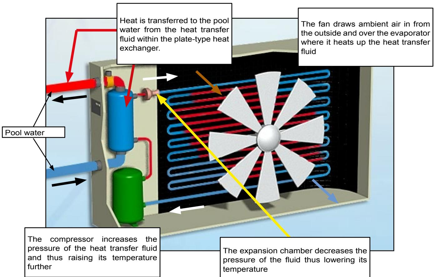
With an ambient air temperature of 15°C, BWT heat pumps transfer 4 to 5 times more energy to the pool water than they consume (90% of this energy is consumed by the compressor): these machines have a yield (or COP - Coefficient of Performance) of between 4 and 6.
