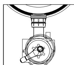
**WASTE :** The water coming from the pump is directed to the waste outlet without passing through the filter.
