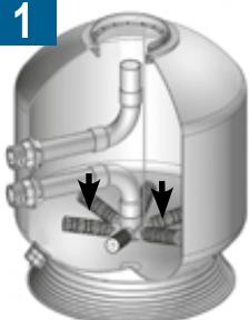
Check along the length of the laterals that they are correctly tightened.
