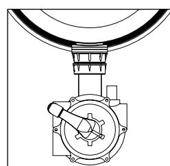
**CLOSED :** No water circulation in this position. Make sure that the pump is never run while in this position.
