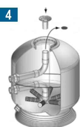
Taking care not to damage the laterals, pour in the load of gravel, followed by the sand. Remove the tape from the collector tube and put back the diffuser.
