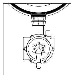
**FILTRATION :** Normal position of the valve. The water coming from the pump passes from the top to the bottom of the filter and then returns to the pool.
