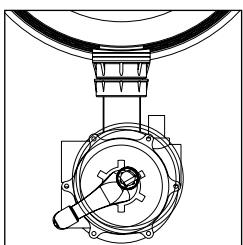
**WASTE :** The water coming from the pump is directed to the waste outlet without passing through the filter.
