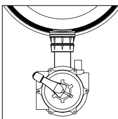
**CLOSED :** No water circulation in this position. Make sure that the pump is never operated in this position.
