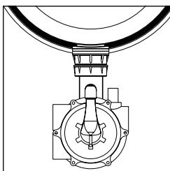
**BACKWASH :** The water coming from the pump passes from the bottom to the top of the filter to escape through the waste outlet washing away the impurities retained by the filter.
