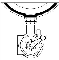
**RECIRCULATE :** The water coming from the pump is directed to the pool without passing through the filter.
