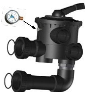
Mount the multi-port valve. Connect the lower bulkhead fitting and then the upper bulkhead fitting. Tighten the nuts moderately
