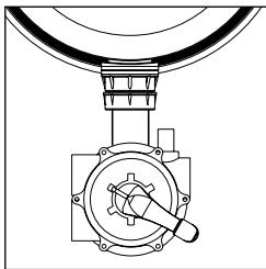
**RINSE :** The water coming from the pump passes from the top to the bottom of the filter and escapes through the waste outlet.
