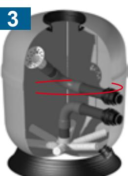
Pour the sand (granulometry 0.6/1.25) in carefully to avoid damaging the laterals.
