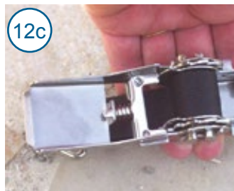
12c Raise the buckle to create enough slack to unhook the strap.
