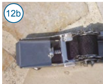
12b Flip the grip 180° while compressing the spring to release the buckle.
