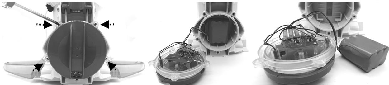
2. To detach the battery connection wire, press on the clip of the connector to pull it out. NOTE: Wrap the connector immediately with insulating tape in order to avoid any short circuit caused by the contact of both wire terminals.
